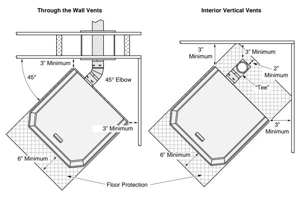
**Note**: If interior vertical pellet vent is used, the clearance to the backwall is determined by the upward-turning elbow or "Tee". It will vary in depth depending on the brand of pellet vent used (it is approximately 5"). Before placing the heater, connect the elbow or "Tee" and measure off the 3" clearance.
